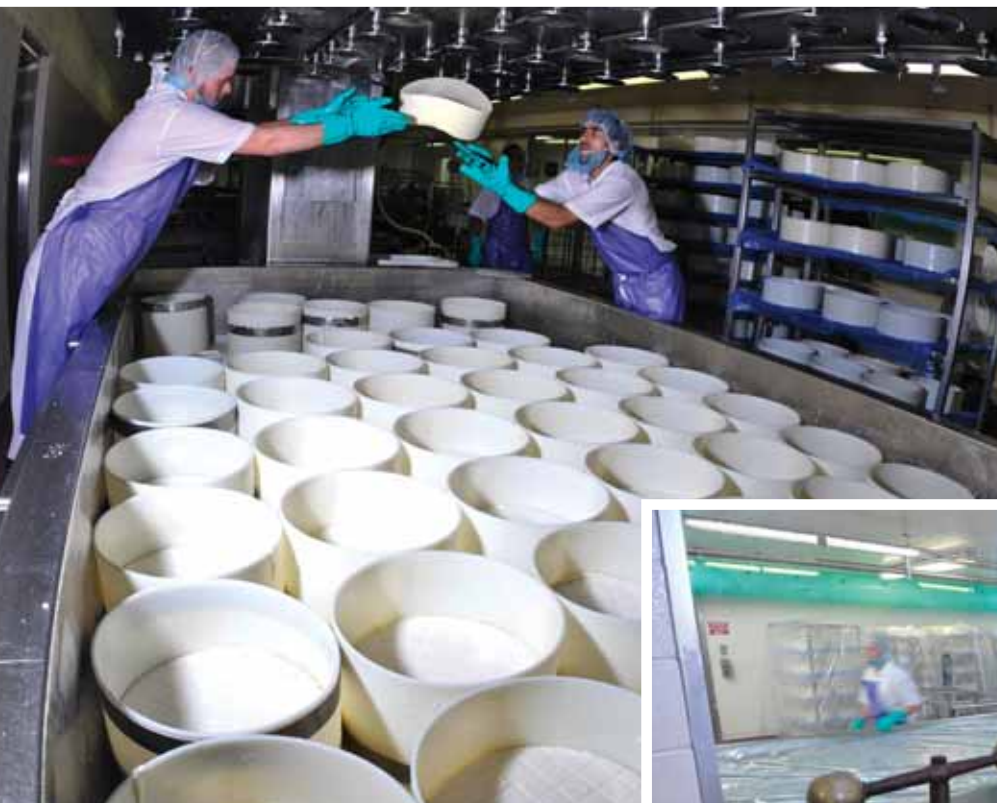
■ (Left) Gruyère is hand flipped during a pause in machine pressing. (Below) The plant's viewing hall features vintage cheesemaking tools and company artifacts. (Bottom) QC Manager Kevin Davis tests racked cheese headed for brine operations.
